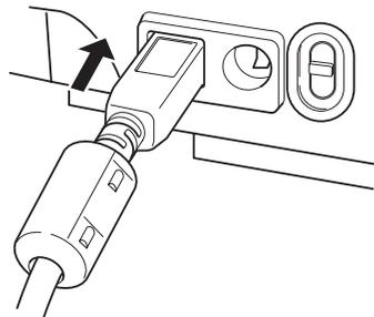
Communication interface in this instrument conforms to USB1.1.
