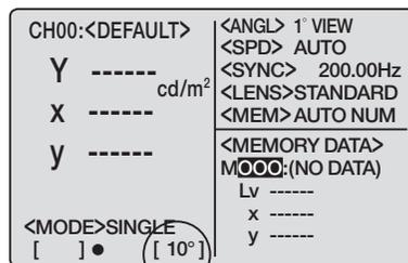
When field of view is set to 10°, Lv display changes to Y display. Lv and Y display in stored data is retained after changing field of view.
