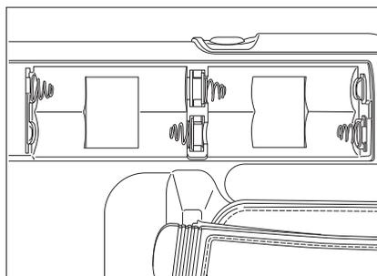
3. Place 4 AA size batteries following polarity indication in battery chamber.
