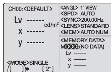
2. Press **SHIFT** to switch to **SHIFT** mode. **[SFT]** appears on bottom left of measurement screen. Or make sure that **[SFT]** appears on left bottom indicating that this instrument has been operated in SHIFT mode.
