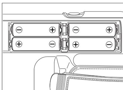
4. Slide battery chamber cover to the direction shown in illustration and close until clicking.
