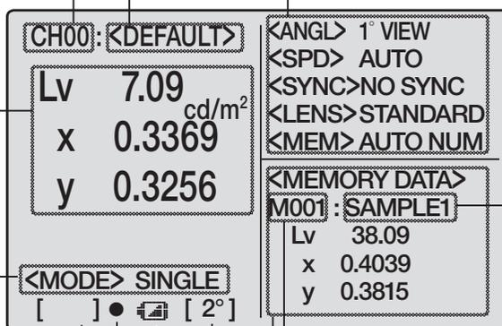
SINGLE is displayed when the measurement mode is set to "Single measurement"; CONT. is displayed when set to normal screen for "Continuous mode". (p.44)
