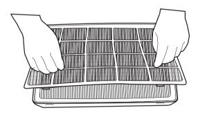
5. Pull the belts on both sides lightly, and HEPA filters can be took out easily.
