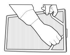
2. Hold the front edge of the filter, insert the protruding parts of the filter into the slot on filtration system side, and then bend the other side, the pre-filter to be fully loaded.
