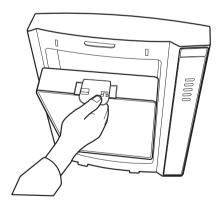
4. Install the bottom clip of front cover to the clip base of fuselage, then push upper end gently to fix the cover.
