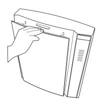
3. Pinch filtration system under the pressure to prominent positions, remove the entire filter system.
