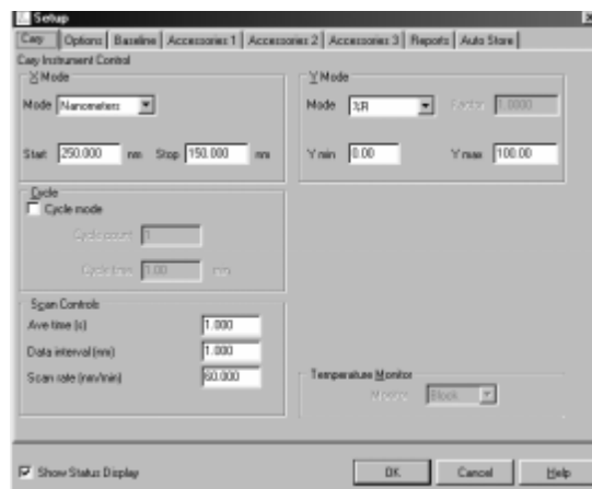
Figure 3. Instrumental parameters for optical coating measurement
