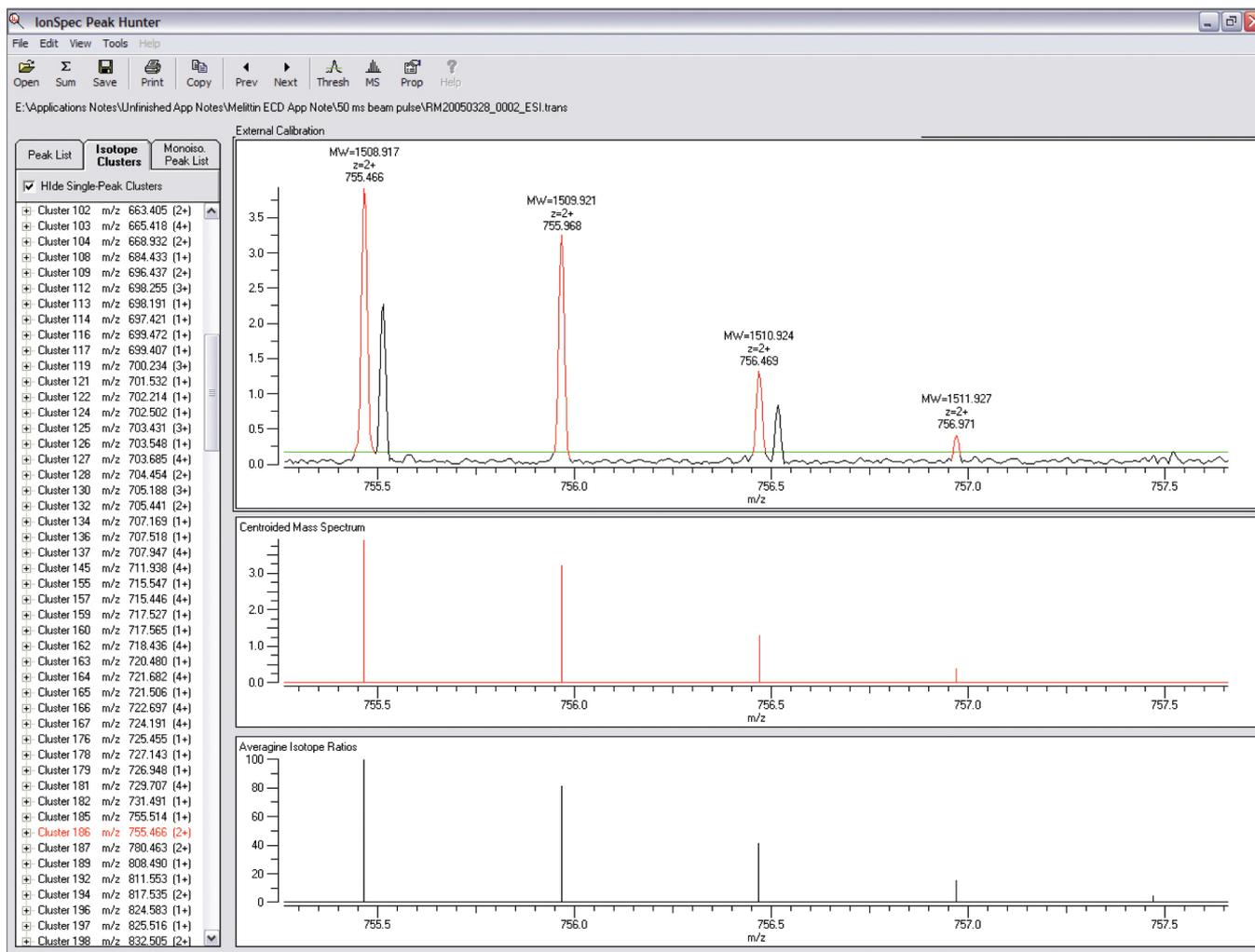
Figure 4 PeakHunter™ software interrogates the complex MS/MS spectrum of melittin to accurately identify isotope clusters.
