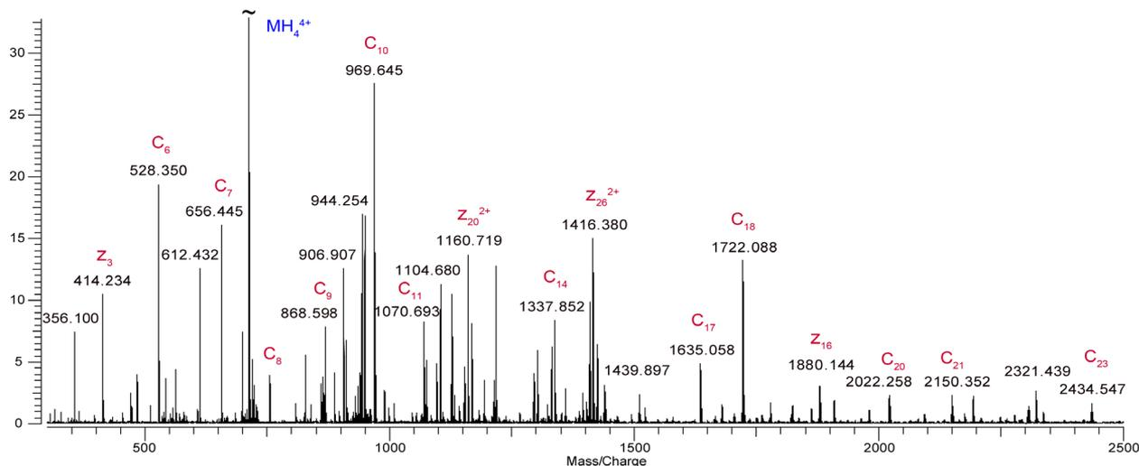
Figure 2 Quadrupole isolation and ECD fragmentation of the +4 charge state of melittin ( $m/z$  712) using a 50 ms electron beam pulse.
