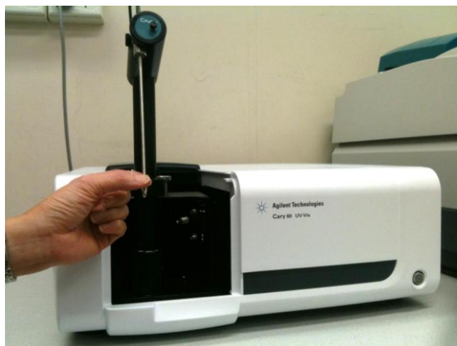
Figure 1. The Cary 60 instrument fitted with the Fiber Optics Accessory taking a reading of 150 µL DNA in an Eppendorf tube at 4 °C
