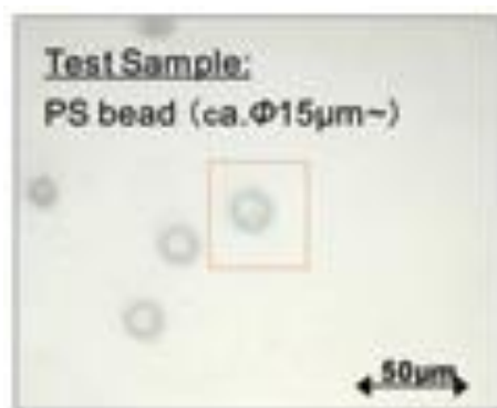
Figure 5. Visible image of a number of polystyrene beads known to have an approximate diameter of 15 \mu\text{m}
