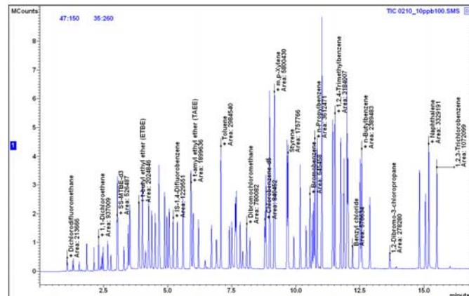
Figure 2. TIC for all target compounds. Excellent peak shape, resolution and sensitivity were easily obtained with the Varian FactorFour™ VF-624ms column and 240-MS GC/MS.
