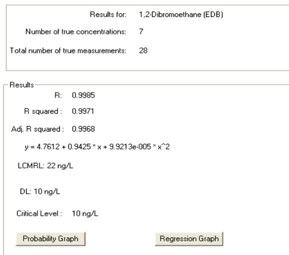
Figure 4b. Results for EDB. LCMRL is calculated to be 22 ng/L, with a predicted detection limit (DL) of 10 ng/L.
