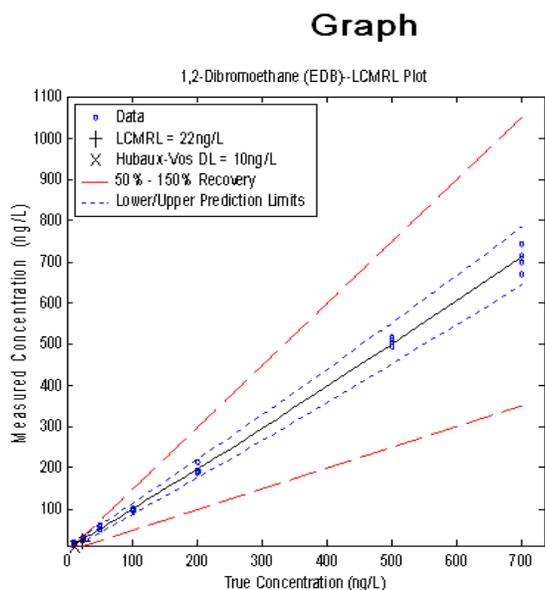
Figure 4a. Calibration curve regression graph for EDB obtained as output from the LCMRL calculator.
