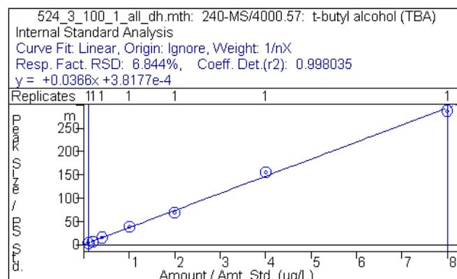
Figure 3. Calibration curve for t-butyl alcohol (TBA) from 0.5 to 40 ppb. Although typically a very poor purge-and-trap compound, it shows excellent response on the 240-MS GC/MS.
