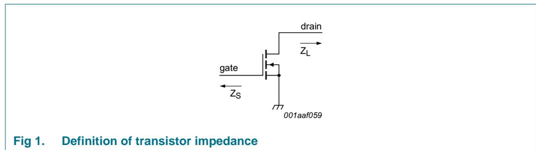
**Fig 1. Definition of transistor impedance**
