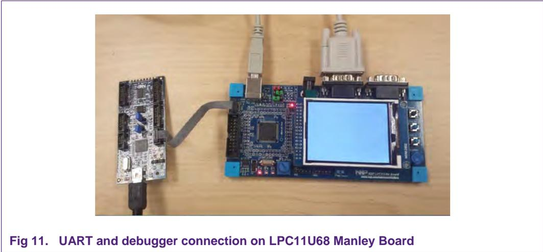
For the Keil IDE use the ULINK debugger, for LPCXpresso IDE use the LPC Link-2 and for IAR Embedded Workbench IDE the Jlink can be used.
