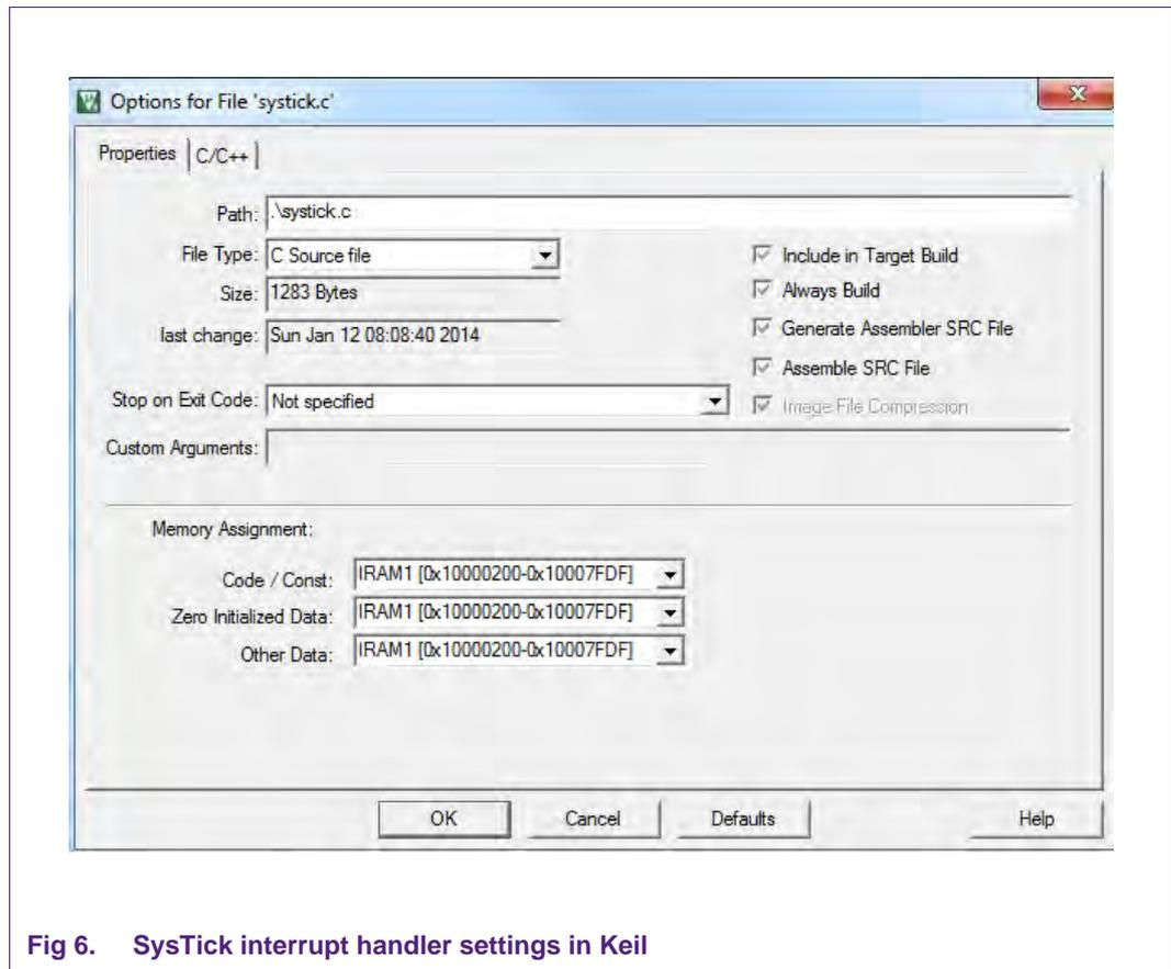
Fig 6. SysTick interrupt handler settings in Keil
