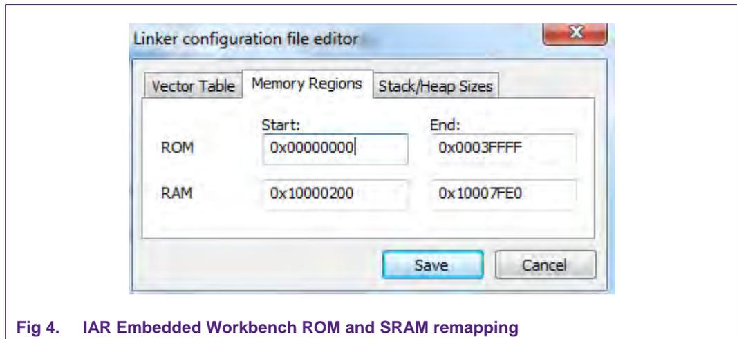
Fig 4. IAR Embedded Workbench ROM and SRAM remapping
