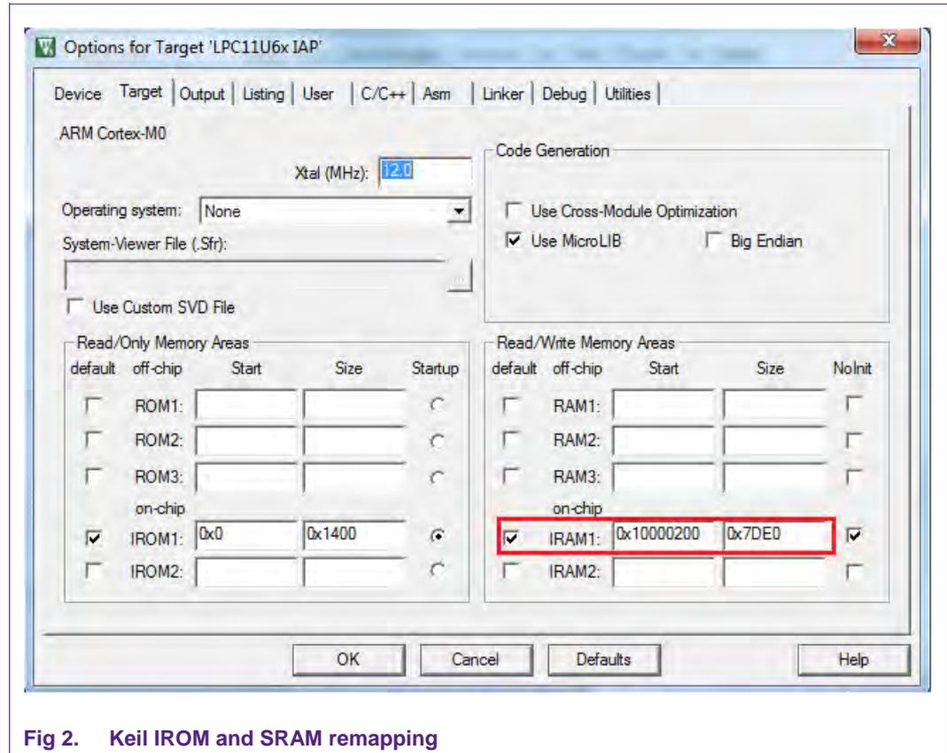
Fig 2. Keil IROM and SRAM remapping
