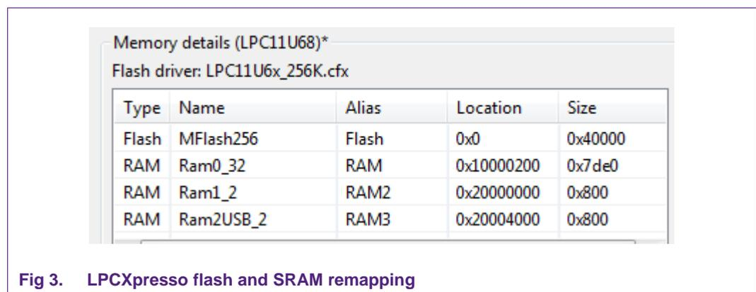
Fig 3. LPCXpresso flash and SRAM remapping
