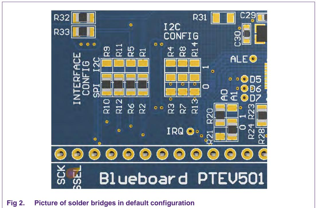
Fig 2. Picture of solder bridges in default configuration
