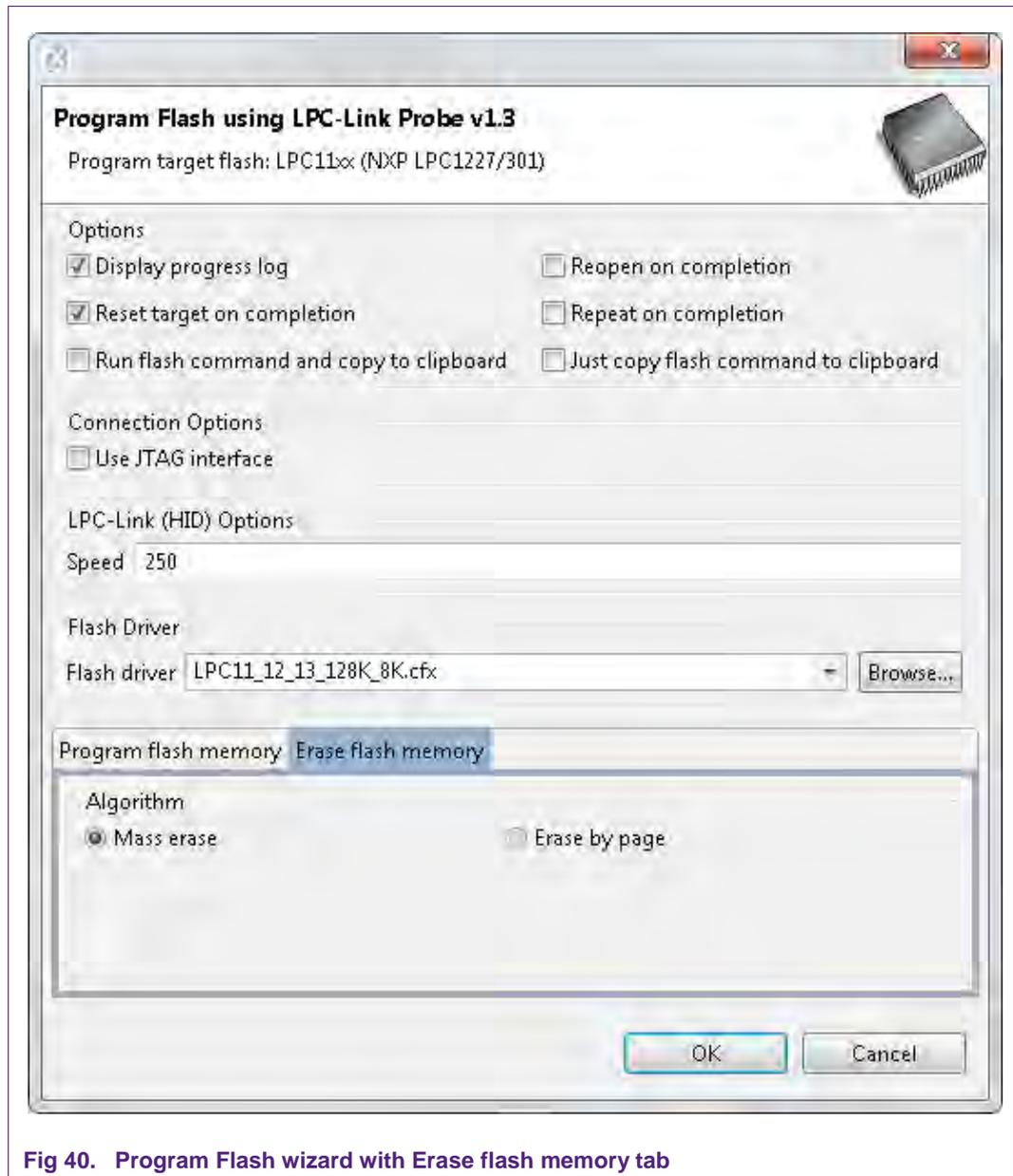
Fig 40. Program Flash wizard with Erase flash memory tab
