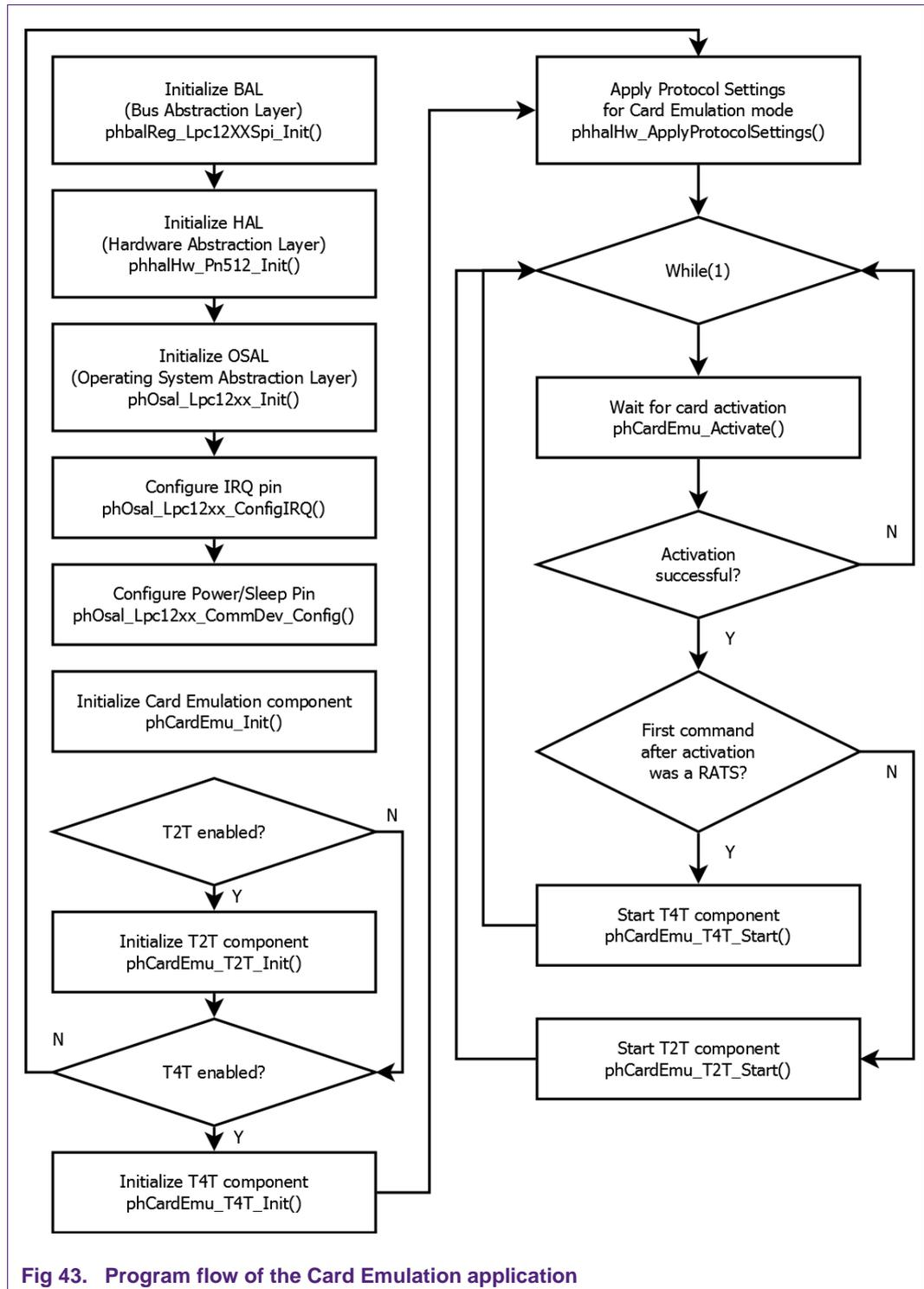
Fig 43. Program flow of the Card Emulation application
