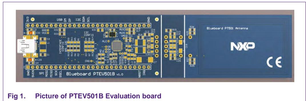
Fig 1. Picture of PTEV501B Evaluation board
