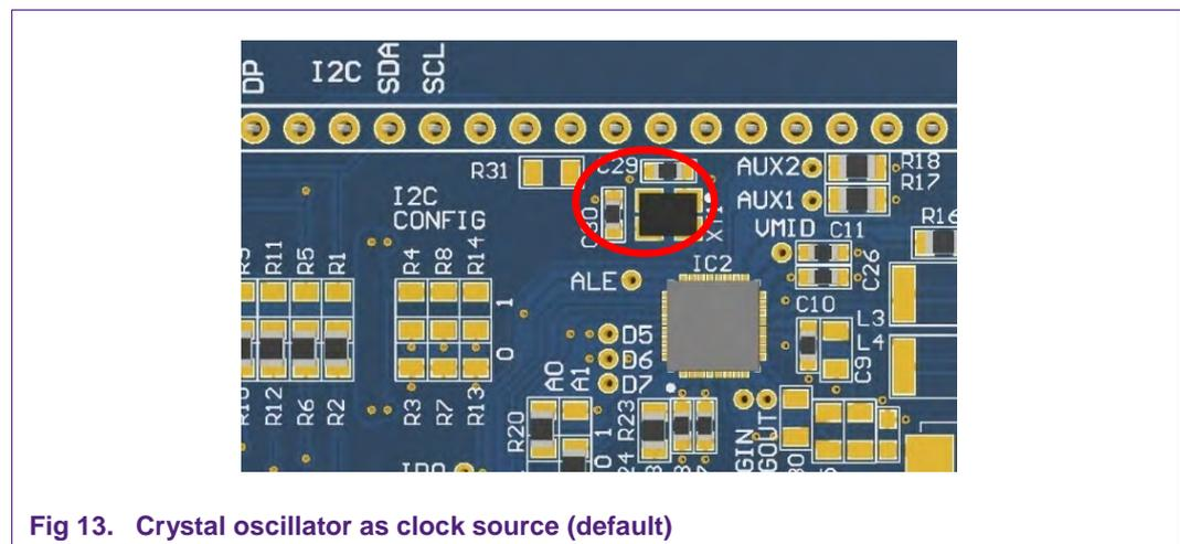
**Fig 13. Crystal oscillator as clock source (default)**
