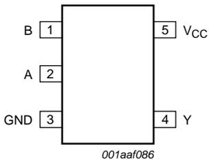
Fig 4. Pin configuration
