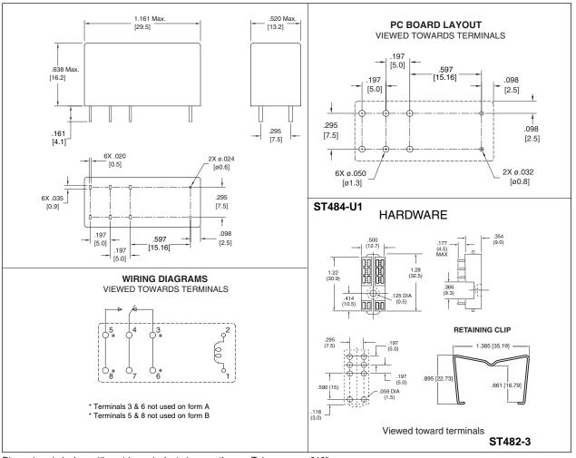
Dimensions in inches with metric equivalents in parentheses. Tolerance:  $\pm .010$ "
