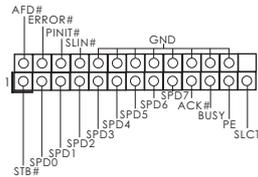
This is an interface for print port cable that allows convenient connection of printer devices.
