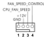
Please connect the CPU fan cable to this connector and match the black wire to the ground pin.
