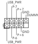
Besides four default USB 2.0 ports on the I/O panel, there are two USB 2.0 headers on this motherboard. Each USB 2.0 header can support two USB 2.0 ports.
