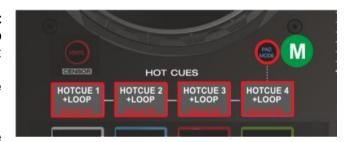
The LED of the Pad will turn red if the HotCue is assigned and will flash while the loop is triggered.
