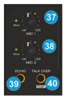
**40. TALK OVER.** Use this button to enable/disable **Talk Over** (led will blink when engaged). When enabled, the MC4000 detects the MIC inputs and attenuates the audio signal level of the master output. When using the microphone, this function prevents the microphone audio from being covered by the music, making speech easier to hear
