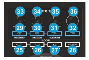
Hold **SHIFT** down and then use this button to set a **Loop In** (Entry) point for manual looping.
