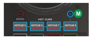
Hold **SHIFT** and then press any of the 4 Pads to **delete** its assigned Hot Cue Point.
