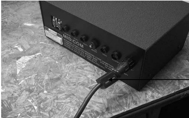
Figure 3. Ferrite Cylinder Clamp Installation
