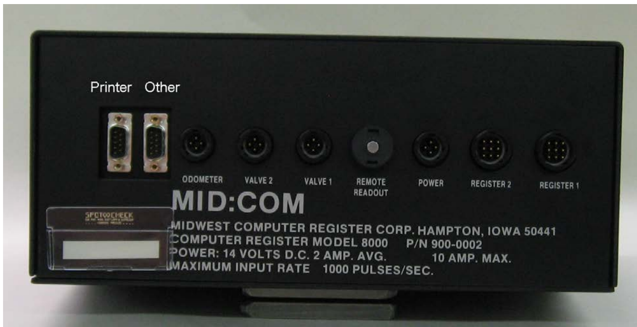
Figure 2. 8000 Back Panel Including Serial Ports
