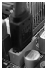
Connect the SATA data cable to the eSATAII connector (eSATAII_TOP)
