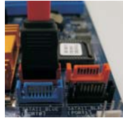
Connect the SATA data cable to the red SATAII connector (SATAII_RED (PORT2))
