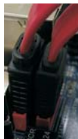
Connect the SATA data cables to both red eSATAII connector (eSATAII_BOTTOM) and orange eSATAII connector (eSATAII_TOP)
