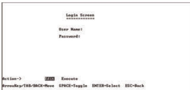
Press the **Esc** button and you will return to the login screen. Use the right arrow button to navigate to **Execute** and press the **Enter** button to enter the CLI interface.
