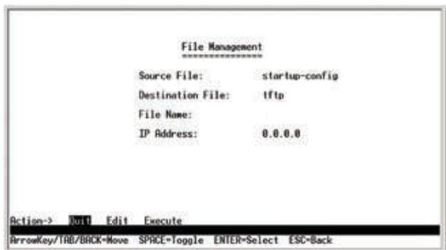
Select **Edit** to change the settings. When your changes are complete, press the **Esc** key to return to the Action menu, and select **Execute** to upload or download the designated file. After you download a new image file, the device should be rebooted.
