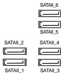
These six Serial ATAII (SATAII) connectors support SATAII or SATA hard disk for internal storage devices. The current SATAII interface allows up to 3.0 Gb/s data transfer rate.
