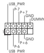
Besides six default USB 2.0 ports on the I/O panel, there are three USB 2.0 headers on this motherboard. Each USB 2.0 header can support two USB 2.0 ports.
