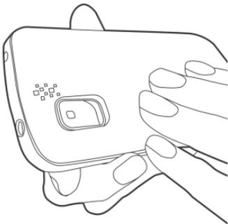
2. Then, press the bottom of the back cover until click into place.
