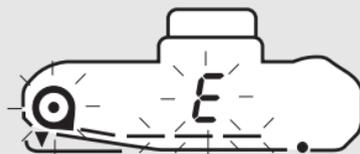
Display signaling film-loading-error
