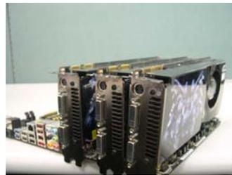
Step2. Connect the auxiliary power source to the PCI Express graphics card. Please make sure that both power connectors on the PCI Express graphics card are connected. Repeat this step on the three graphics cards.
