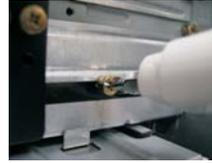
**Step 5** Plug the Front USB 3.0 cable into the USB 3.0 header (USB3\_4\_5 or USB3\_6\_7) on the motherboard.
