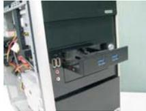
**Step 4** Screw the Front USB 3.0 Panel to the drive bay with six chassis screws.
