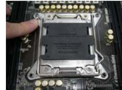
Step 1-2. Disengage the right lever by pressing it down and sliding it out of the hook.
