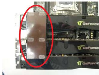
Step4. Connect a VGA cable or a DVI cable to the monitor connector or the DVI connector of the graphics card that is inserted to PCIE1 slot.
