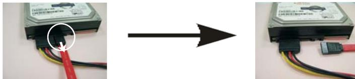
**Step 2** Unplug SATA 15-pin power cable connector (Black) from SATA / SATA2 / SATA3 HDD side.
