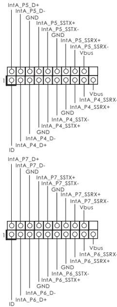
Besides two default USB 3.0 ports on the I/O panel, there are two USB 3.0 headers on this motherboard. Each USB 3.0 header can support two USB 3.0 ports.
