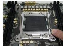
Step 1-3. Keep the right lever positioned at about 90 degrees in order to flip up the load plate.
