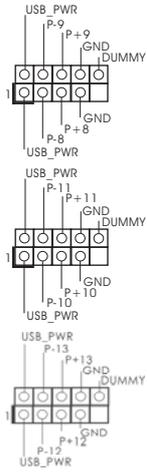
Besides six default USB 2.0 ports on the I/O panel, there are three USB 2.0 headers on this motherboard. Each USB 2.0 header can support two USB 2.0 ports.
