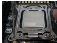
Step 3-3. Press down the left load lever, and secure it with the load plate tab under the retention tab.
