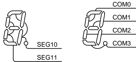
Figure 15-5 Example of COM, SEG Pin Connection (1/4 duty)
