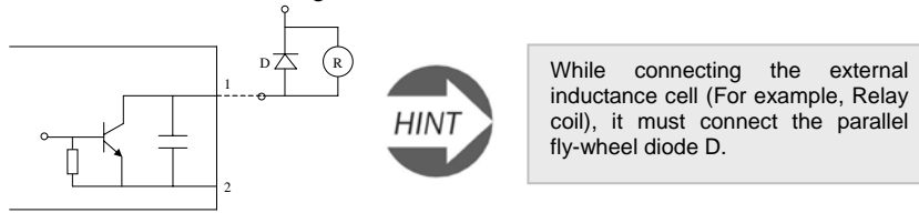
Fig.6-12 Inner wiring diagram of output terminals
