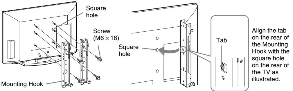
Align the tab on the rear of the Mounting Hook with the square hole on the rear of the TV as illustrated.
