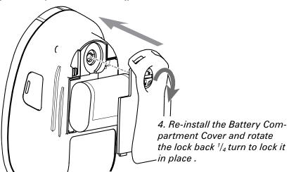
Ensure battery leads are not pinched prior to replacing battery cover.
