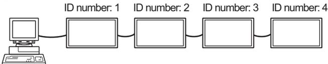
If monitors are connected as shown above, you can execute commands like "Set the volume of the monitor with ID 4 to 20".
