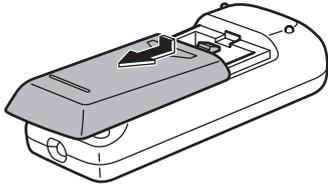
2. See the instructions in the compartment and put in the batteries (R-6 ("AA" size) x 2) (supplied with the PN-ZR01 (optional)) with their plus (+) and minus (-) sides oriented correctly.
