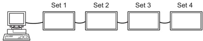
\* If monitors are connected as shown above, you can execute a command like "Set all monitors' input settings to PC D-SUB".
