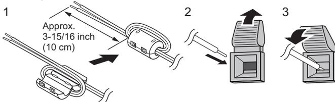
1. Attach a speaker cable core (included with the PN-ZB02) to the end of the speaker cable connected to the monitor.
