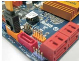
Connect the SATA data Cable to the orange SATAII connector (SATAII_6)
