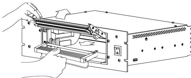
从打印机上取出打印纸托架，从托架上取出纸杆，从纸杆上抽出空纸筒。
