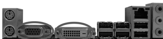
VGA/D-Sub port VGA/DVI-D port
