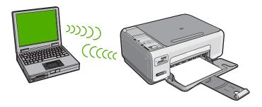
In order to connect the HP All-in-One to your computer (ad hoc), you need to create an ad hoc network profile on your computer. This includes choosing a network name (SSID) and WEP security (optional but recommended) for your ad hoc network.
