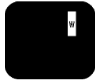
Three adjacent lit subpixels (one white pixel)
