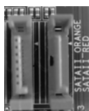
SATAII_RED (PORT 1) and SATAII_ORANGE (PORT 2)
