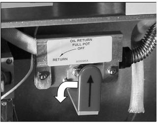
5. The cooking oil/shortening is pulled through the filter and pumped up to and through the Power Shower, finally returning to the filter pan through the open frypot-drain.
