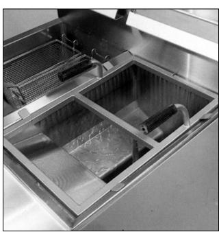
6. After the oil is filtered, close the drain valve and allow the fryer to refill.
