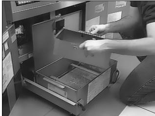
2. Remove the paper hold-down ring (and if changing the filter paper, remove and discard the used filter paper). Remove the filter screen and clean the crumb tray, hold-down ring, filter screen, and pan with a solution of hot water and dishwashing detergent, ensuring that all breading and food particles are removed from the pan. Ensure the pan is dried completely. Allow the screen to dry completely before reinstalling.
