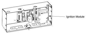
Depending upon when the unit was manufactured, full vat units may have either one or two ignition modules. If there is only one ignition module, the fuse will be mounted on the interface board.
