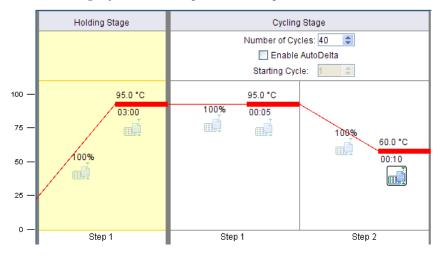
Run the PCR1Place the reactions in the StepOnePlus instrument.Program2On the Run screen, click START RUN.
