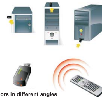
3 CIR sensors in different angles
