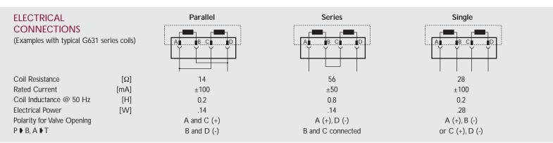
Note: Before applying electrical signals, the pilot stage must be pressurized.
