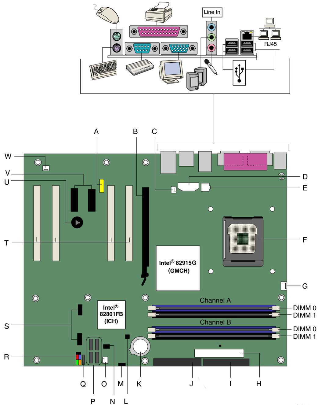
Figure 1. Desktop Boards D915GAV and D915GEV Components
