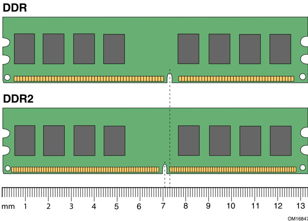
Figure 17. Matching the Correct DIMM
