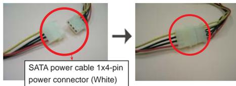
SATA power cable 1x4-pin power connector (White)
