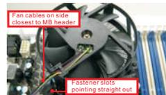
Step 3. Align fasteners with the motherboard through-holes.
