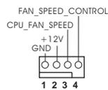
Please connect the CPU fan cable to the connector and match the black wire to the ground pin.
