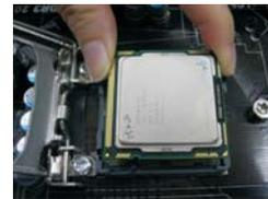
Step 3-4. Verify that the CPU is within the socket and properly mated to the orientation keys.
