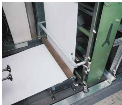
ELROLLER SRS 41 on flexo printing machine
