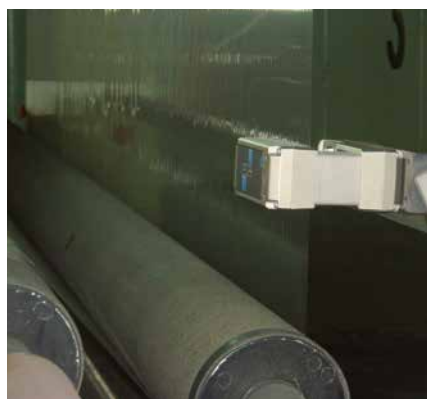
Ultrasonic edge sensor FX 5 in film manufacturing machine
