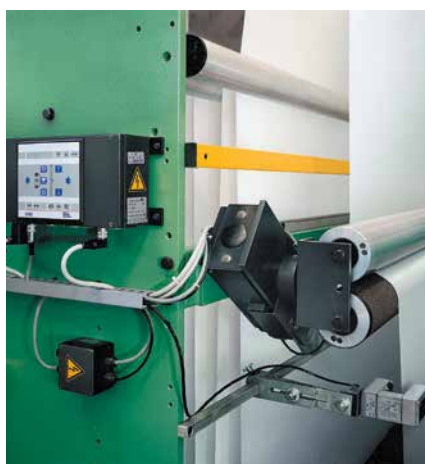
ELROLLER VGS 14 on bag making machine
