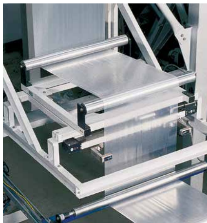
ELGUIDER DRS 31 on blow film extruder
