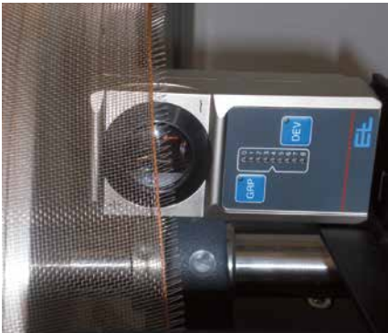
Infrared edge sensor FR 52 for mesh acquisition
