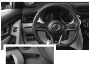
Lock the steering wheel in place by pushing the lock lever up firmly.
