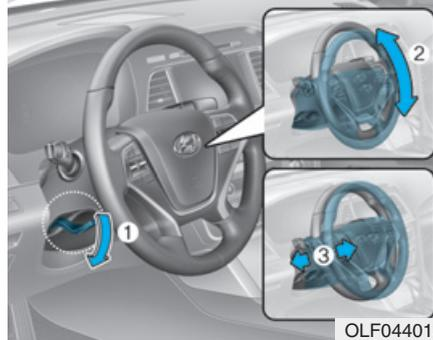
Pull down the lock-release lever (1) on the steering wheel column and adjust the steering wheel angle (2) and position (3, if equipped). Move the steering wheel, so it points toward your chest, not toward your face. Make sure you can see the instrument panel warning lights and gauges.
