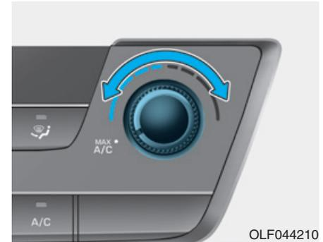
The temperature control knob allows you to control the temperature of the air flowing from the ventilation system. To change the air temperature in the passenger compartment, turn the knob to the right position for warm and hot air or left position for cooler air.
