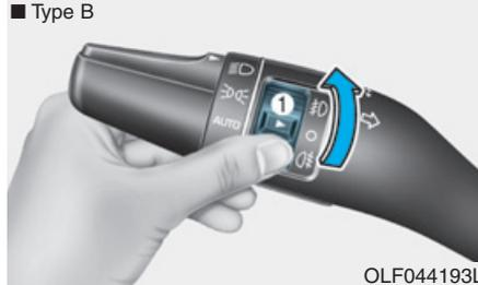
Fog lamps are used to provide improved visibility when visibility is poor due to fog, rain or snow, etc. Use the switch next to the headlamp switch to turn the fog lamps ON and OFF.
