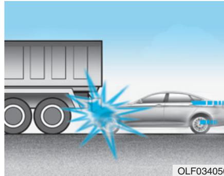
Just before impact, drivers often brake heavily. Such heavy braking lowers the front portion of the vehicle causing it to “ride” under a vehicle with a higher ground clearance. Air bags may not inflate in this “under-ride” situation because deceleration forces that are detected by sensors may be significantly reduced by such “override” collisions.
