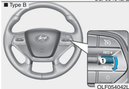
3. Push the lever (1) down (SET-), and release it. The SET indicator light will illuminate.
