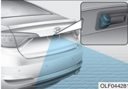
The Rear View Camera will activate when the engine is running and the shift lever is in the R (Reverse) position.
