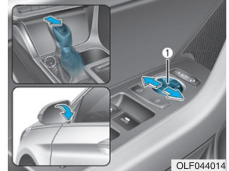
When you move the shift lever to the R (Reverse) position, the outside rearview mirror(s) will rotate downwards to aid with driving in reverse.
