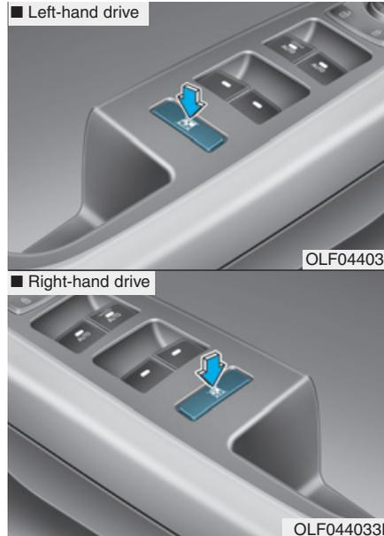
The driver can disable the power window switches on the rear passengers' doors by pressing the power window lock switch.
