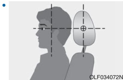
Adjust the headrests so the middle of the headrests is at the same height as the height of the top of the eyes.
