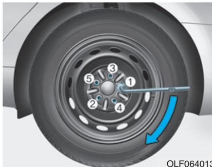
14. Use the wheel lug nut wrench to tighten the lug nuts in the order shown. Double-check each lug nut until they are tight. After changing tires, we recommend that an authorized HYUNDAI dealer tighten the lug nuts to their proper torque as soon as possible. **The wheel lug nut should be tightened to 9~11 kg.m (65~79 lb.ft).**
