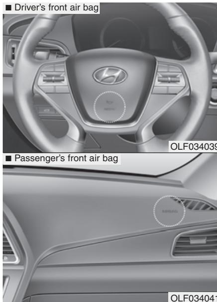
The purpose of the SRS is to provide the vehicle's driver and front passengers with additional protection than that offered by the seat belt system alone in case of a frontal impact of sufficient severity.
