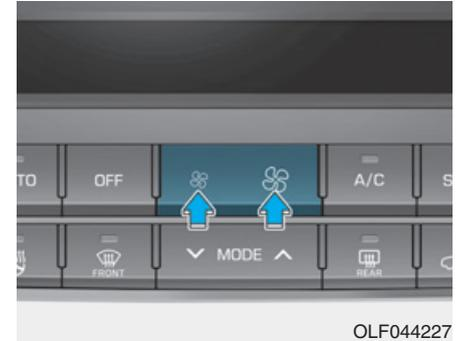
The fan speed can be set to the desired speed by pushing the fan speed control button.
