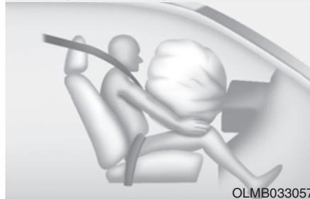
After complete inflation, the air bag immediately starts deflating, enabling the driver to maintain forward visibility and the ability to steer or operate other controls.
