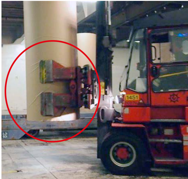
Picture 8. Visual sliding signs of too low clamping force
