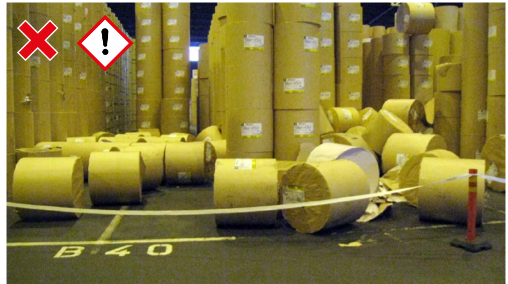
Picture 14. Example of reel collapsing accident.
