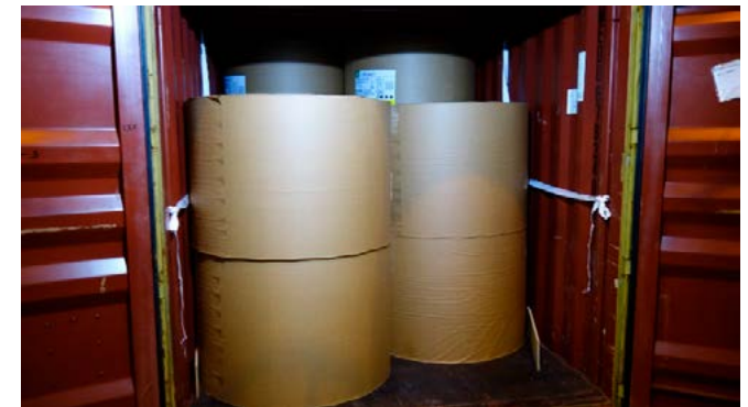
Hardboard used as a protection material in containers
