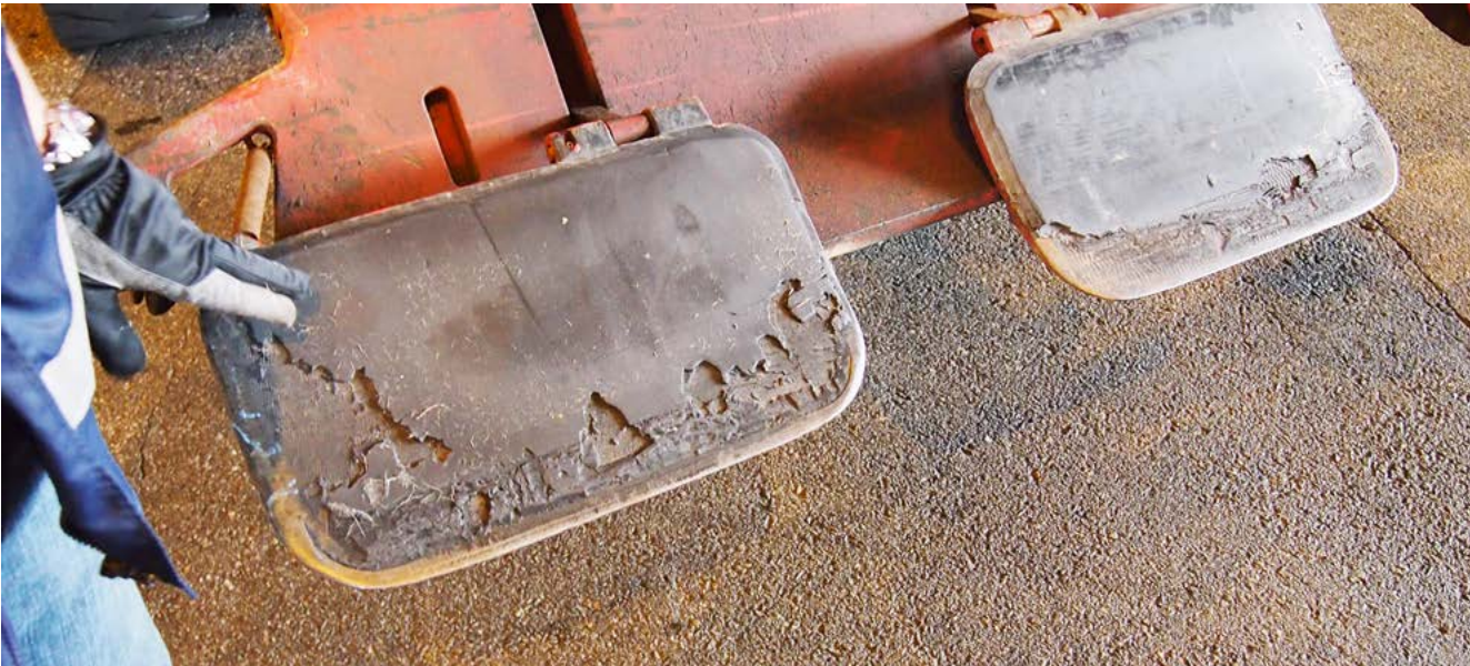
Picture 4. Poor condition of clamp pad friction material.
