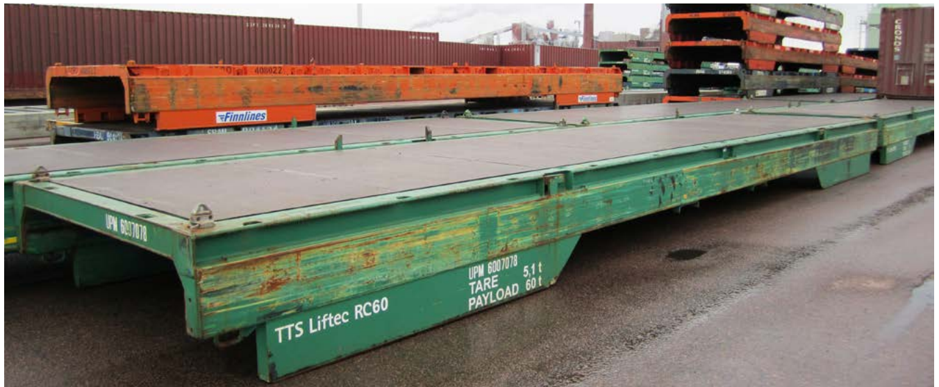
Cassette (12x2,6x0,9 meters, tare 5,5 tons, safe working load 60–80 tons)
