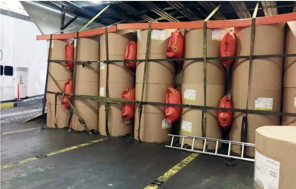
Picture 24. Proper cargo securing in vessel hold.
