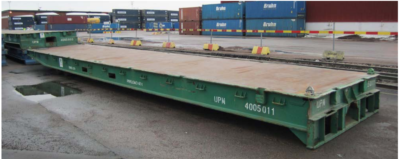
Mafi/roll trailer (12x2,5x0,8 meters, tare 8 tons, safe working load 60–100 tons)
