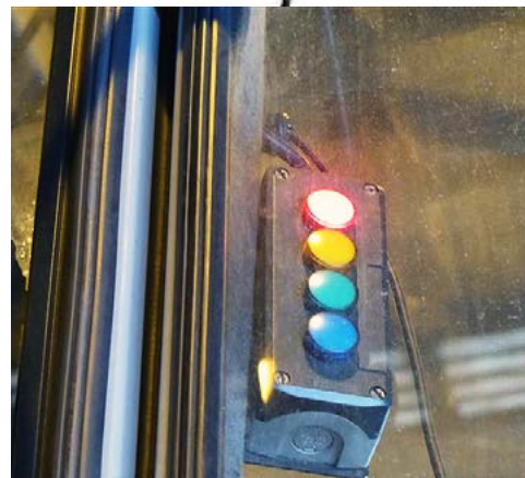
Picture 6. Proper label of compression force pre-setting with indicator lights.
