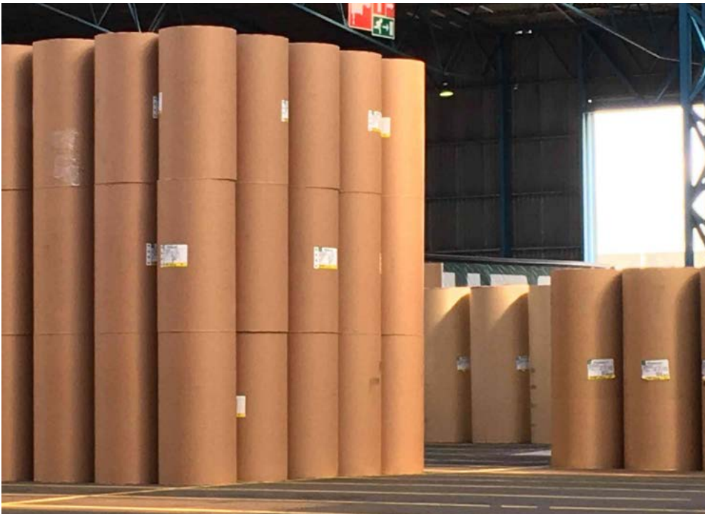
Picture 17. Proper reel stacking in port warehouse
