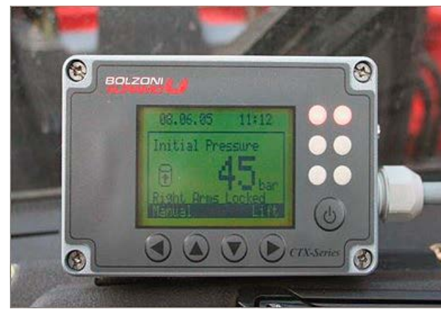
Picture 7. CTX Intelligent clamp screen inside the cabin (source: Bolzoni Auramo).
