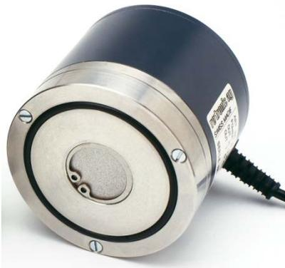
The sensors of the HC2-AW-USB probe are protected with a wire mesh dust filter held in place by a snap-ring
