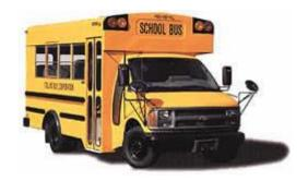
Type B School Bus - A conversion or body constructed and installed upon a van or front-section vehicle chassis or stripped chassis with a gross vehicle weight rating of more than ten thousand (10,000) pounds and designed for carrying more than ten (10) persons. Part of the engine is beneath and/or behind the windshield and beside the driver's seat. The entrance door is behind the front wheels
