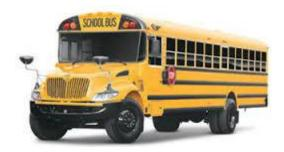
Type D School Bus – A body installed upon a chassis with the engine mounted in the front, midship, or rear with a gross vehicle weight rating of more than ten thousand (10,000) pounds and designed for carrying more than ten (10) persons. The engine may be behind the windshield and beside the driver's seat, at the rear of the bus, behind the rear wheels, or midship between the front and rear axles. The entrance door is ahead of the front wheels
