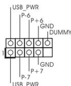
ASRock I/O Plus™ accommodates 6 default USB 2.0 ports. If those USB 2.0 ports on the I/O panel are not sufficient, this USB 2.0 header is available to support 2 additional USB 2.0 ports.
