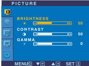
**BRIGHTNESS** Adjusts the brightness of the screen.
