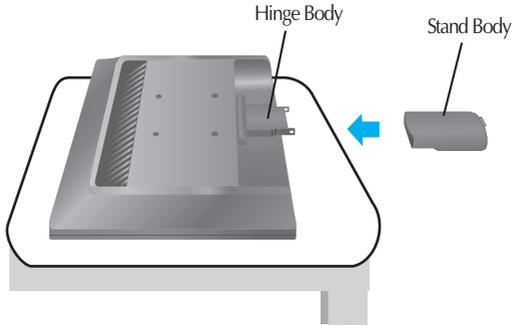
3. Check the direction of the Stand Base, and connect it into the Stand Body.
