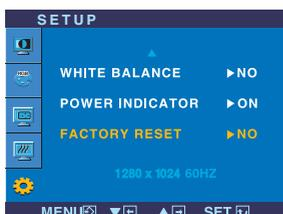
**WHITE BALANCE** If the output of the video card is different the required specifications, the color level may deteriorate due to video signal distortion. Using this function, the signal level is adjusted to fit into the standard output level of the video card in order to provide the optimal image.
