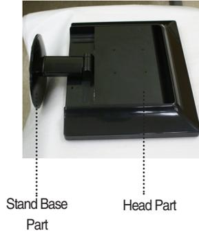
3. Hold the Head Part with one hand and hold the Stand Base Part with the other as shown in the picture and pull the Stand Base Part lightly upward.
