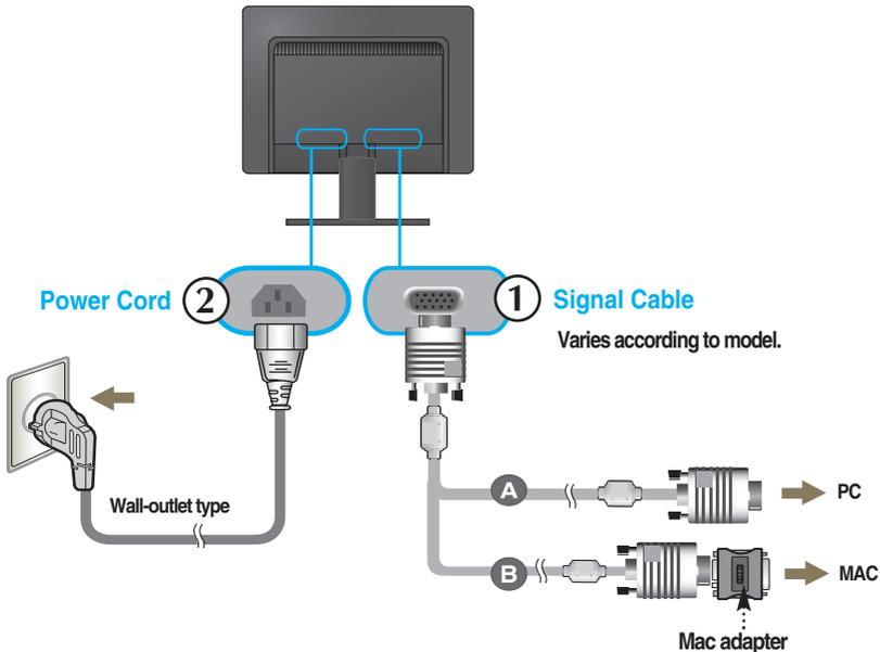
For Apple Macintosh use, a separate plug adapter is needed to change the 15 pin high density (3 row) D-sub VGA connector on the supplied cable to a 15 pin 2 row connector.
