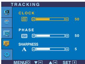
**CLOCK** Adjusts any vertical bars or stripes visible on the screen background. The horizontal screen size will also change.
