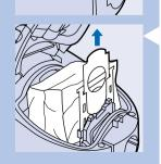
Lift the dustbag out of the compartment by pulling the cardboard lug upwards, which causes the dustbag to be sealed.
