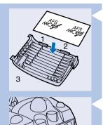
Place the sides (1, 2) and the bottom edge (3) of the new filter properly behind the ridges of the holder.
