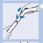
Connect the tubes to each other and to the handgrip by inserting the narrow section into the wider section while turning it a little. The tube with the clip is the lower tube.
