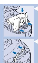
4 Slide the cardboard front of the new dustbag into the two grooves of the dustbag holder. Press it down as far as possible.
