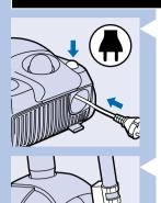
Switch the appliance off and remove the mains plug from the wall socket.
