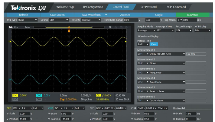
LXI control screen and waveform display enable remote control over Ethernet
