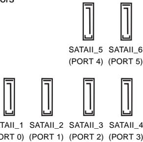
These six Serial ATAII (SATAII) connectors support SATAII or SATA hard disk for internal storage devices. The current SATAII interface allows up to 3.0 Gb/s data transfer rate.
